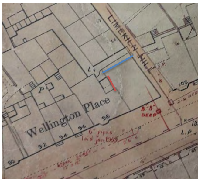
Extract from the Ordnance Survey map at the original scale of 1:500 surveyed in 1891 and published in 1892 The blue line is the north wall which contains the draw arch to the lime kiln The red line is where the side stone wall is also visible in 98 Castle Road Map reproduced courtesy Scarborough Museum and Galleries
